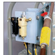
The Millennium pneumatic remote control valve combines inlet and outlet functions.
