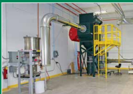
ASHRAE Standard 199 Dust Test Apparatus
