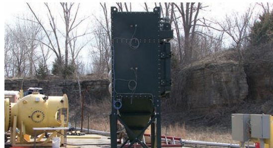
Staged deflagration in cartridge dust collector with explosion venting
