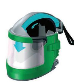
11 Streamlined air system - an even distribution of airflow brings air to the breathe zone and reduces lens fogging. The air channel stops head chill and directs the air where it's needed! Vents in the top dome allow air to also pass around the head for extra comfort. This engineering is supported by a failproof air tube attachment that can only be assembled the correct way, limiting time for re-adjustments and removing the risk of malfunction.
